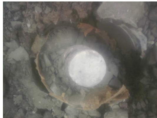
Figure 6-7. Pier 3 (left) and End Abutment (right) test micropiles after load test failure
