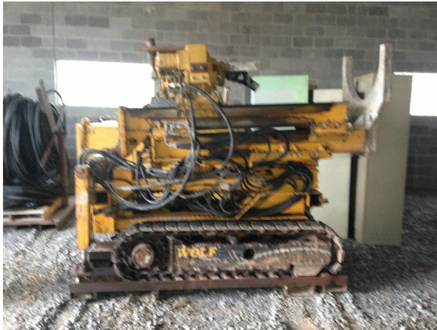
Figure 1-6. Techno Drill 610 compact drill rig
